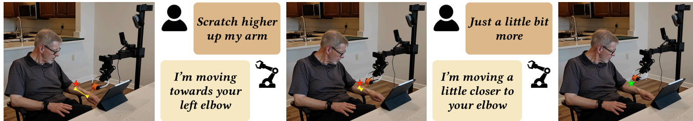
Figure 1: Example interaction with BRIDGE. User is in a scratching scenario, where they command the robot to move to the target scratching position (marked with star) through a bidirectional verbal interaction.
